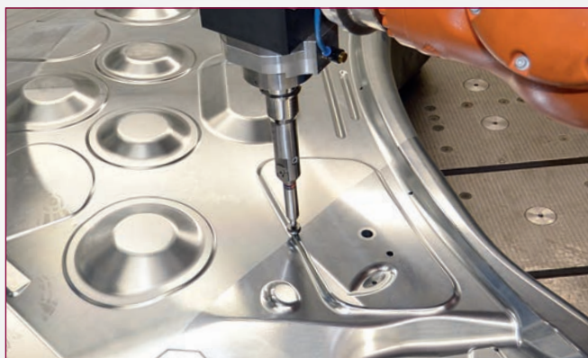
Use of FORGEfix® P for cold forging of batch drawing tools on a robot system
