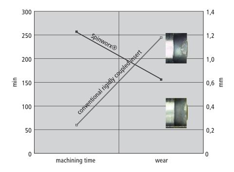
After a machining time of 265 minutes, we have identified a wear land of 0.63 mm for our Spinworx®-inserts. The end of cutting-edge life was still far away.
