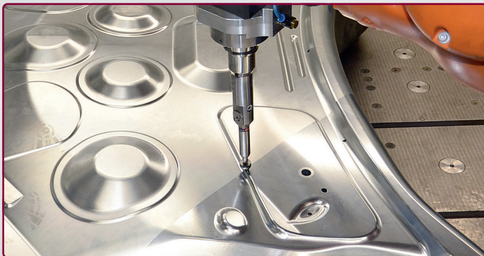
Use of FORGEfix® for cold forging of batch drawing tools on a robot system
